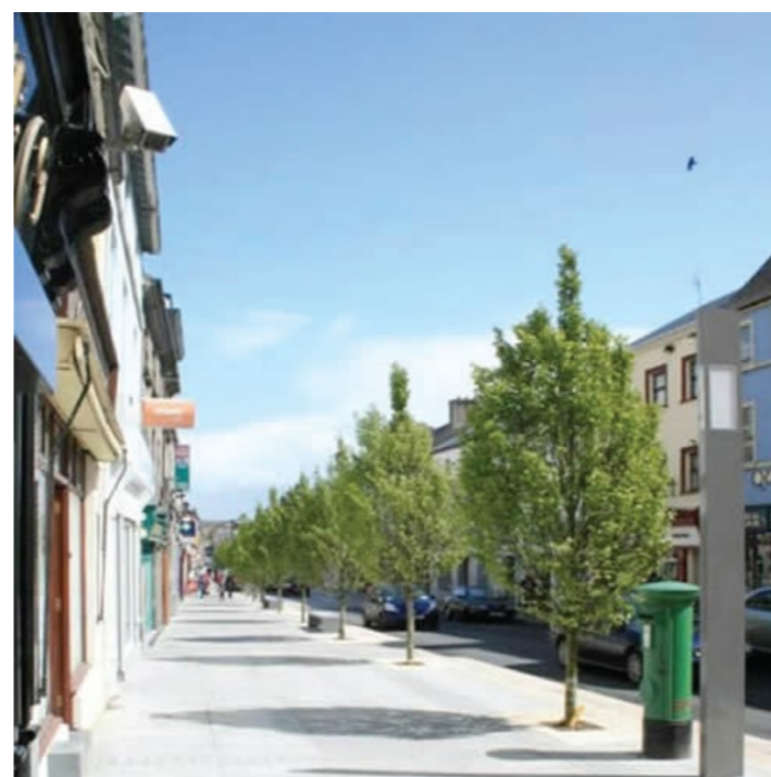
Right: Castlebar Good use of space, proportion and zones. There is a pedestrian zone a car/roadway zone and a transition zone. By aligning the trees, street lights and seating in the transition zone the pedestrian area is free of clutter and easily traversable. The trees soften the space and provide a visual barrier between pedestrians and the car.
